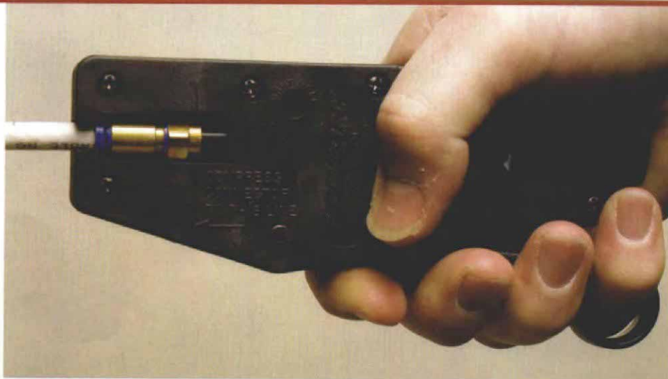
F-connectors terminate RG 6 cable. Having seen a 27-in. TV dangling from one, the author prefers the F-connectors made by Augat (Thomas & Betts; www.tnb.com). These connectors require an Augat IT1000 tool, which costs about $60 but does the entire job from stripping the cable to crimping the F-connector.
